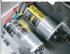
The connecting cables are soldered and the geared motors are now ready for installation in to the model. Please note the additional installation steps in the assembly instructions from the model.
